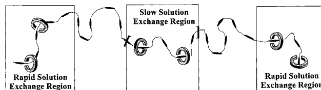
Figure 4. Schematic representation of the extreme cases of exchange rates of threaded macrocyclic components of a polypseudorotaxane with solution. Macrocycles near the ends of the macromolecule undergo rapid exchange on the NMR time scale, while those on host sites located in the interior portions of the linear macromolecule exchange very slowly due to the distance they must traverse and the fact that they cannot pass other threaded macrocycles. In the present systems at ambient temperature macrocycle 1 undergoes rapid exchange with up to ca. three terminal repeat units.
